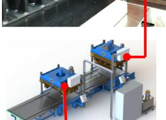
The first station automatically hot-cures the sidewalls onto the base rubber conveyor belt
